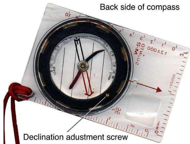
4. **Meridian lines:** Marks on the bottom of the interior of the circular compass housing, marked with parallel 'meridian lines', which rotate with the bezel when it is turned. The meridian lines run parallel to the north-south axis of the bezel, however turned. Meridian lines are necessary for plotting and determining intersections on the map.
