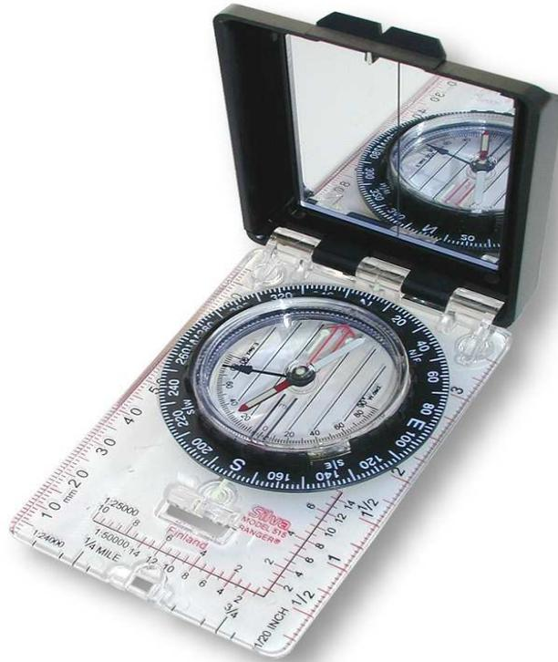
1. **Adjustable Declination:** A move-able orienting arrow, which provides a built-in declination adjustment. If there is one feature which simplifies map and compass work, this is it. Compasses with adjustable declination can often be identified by the presence of an adjustment screw on the back of the housing (on the underside of the compass, look at the bezel - the screw is usually brass or copper colored). Avoid the keyless models!
