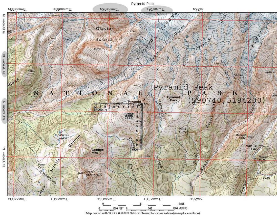
Similarly, the northing is between lines 5184000 and 5185000, between which we interpolate by eye an estimate of 5184200.
