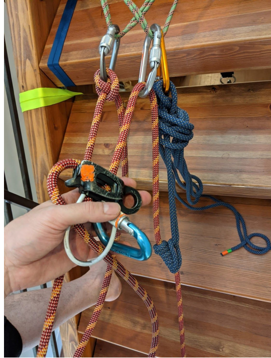
Fig 10. Removing ATC from the anchor.
