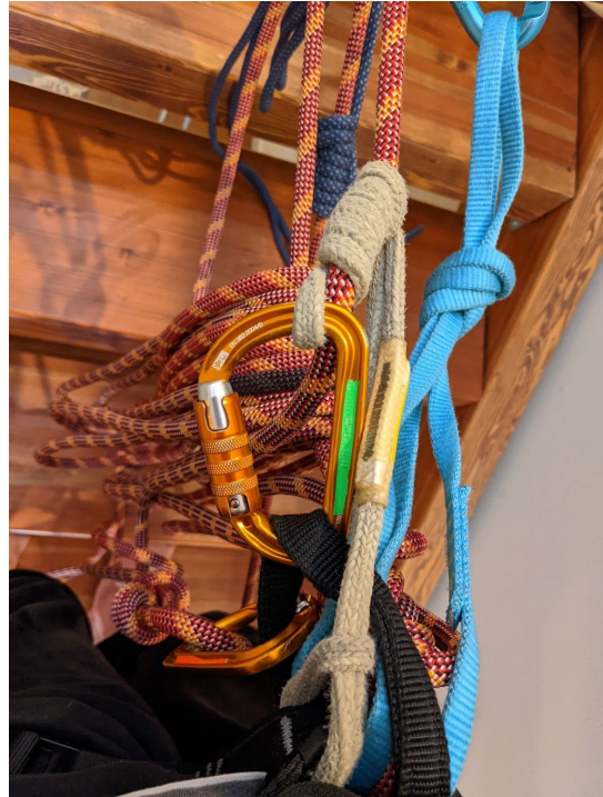
Fig 12. Installing autoblock for rappel.
