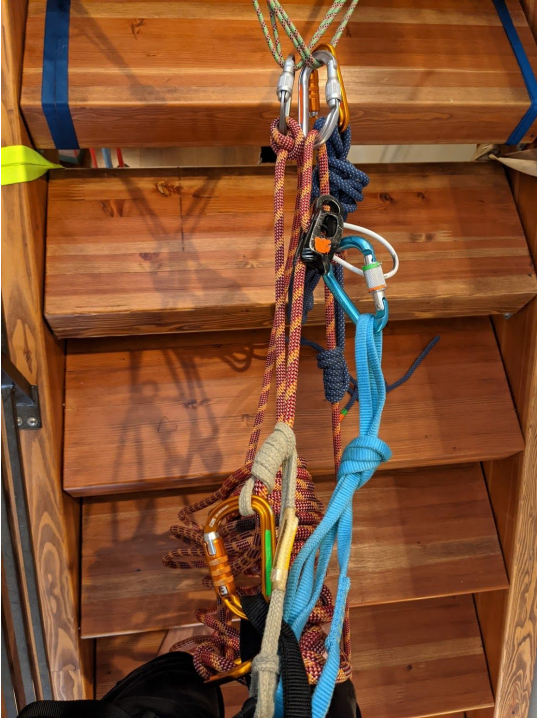
Fig 13. Tensioning the rappel setup.
