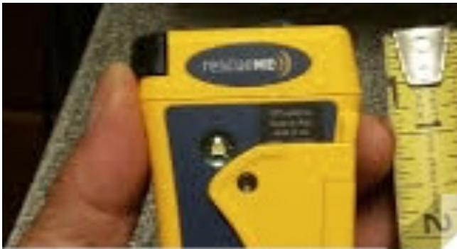
It does not allow any degree of two-way communication like the Garmin InReach variants or the different Spot Messenger devices. It requires registration with NOAA, but there is no subscription required. A mail-in registration form is provided to send to NOAA. Alternatively, NOAA has registration website that is easy to use. When registering essentially you provide the 15-digit device ID and emergency contact information.
