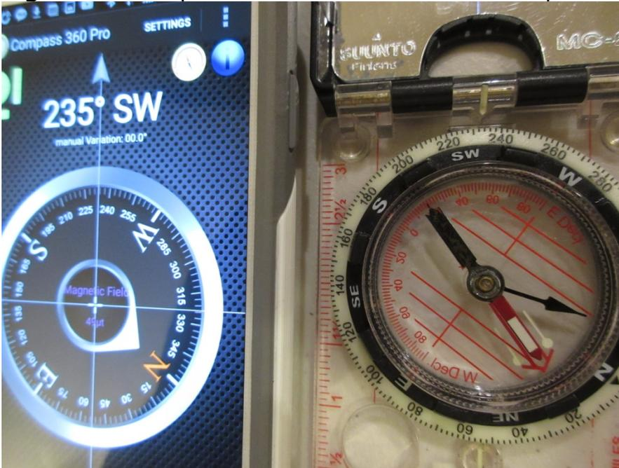
Figure 1 shows the app by itself, and another next to a mechanical compass, showing 235 and 233 degrees respectively, within plus-minus 2 degrees.
