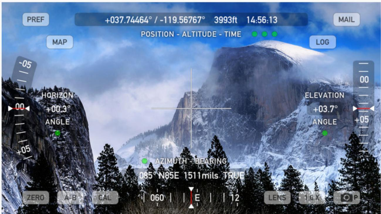
Altimeter GPS Pro 4.0 (<https://itunes.apple.com/us/app/altimeter-gps-pro-elevation/id545185104?mt=8>) provides a simple, bold display of the GPS determined altitude. One touch toggle meters/feet; coordinates only in Lat, Long; compass for cardinal points; auto sunrise/sunset; auto current street address; light/weather/camera; and on trail features; finger swipe displays Open Street Map (OSM) of current position. Cost: Free or \$0.99. --Editor
