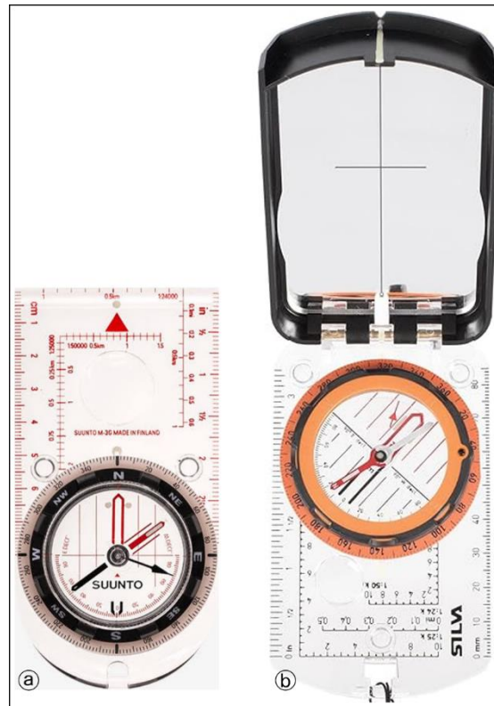
Fig. 3-1. An analog baseplate compass with declination adjustment is highly recommended. The addition of a global needle is suggested. Example compass types: a, analog baseplate compass; b, analog baseplate compass with sighting mirror.
