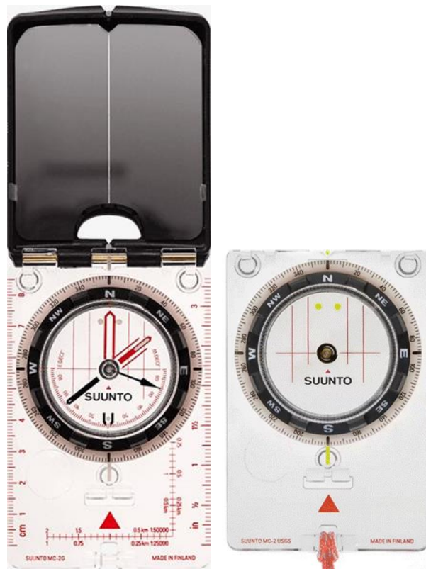
Fig. 3-12. The mirrored compass (a) is reimaged (b) with only the parts essential for measuring or plotting bearings on a map.
