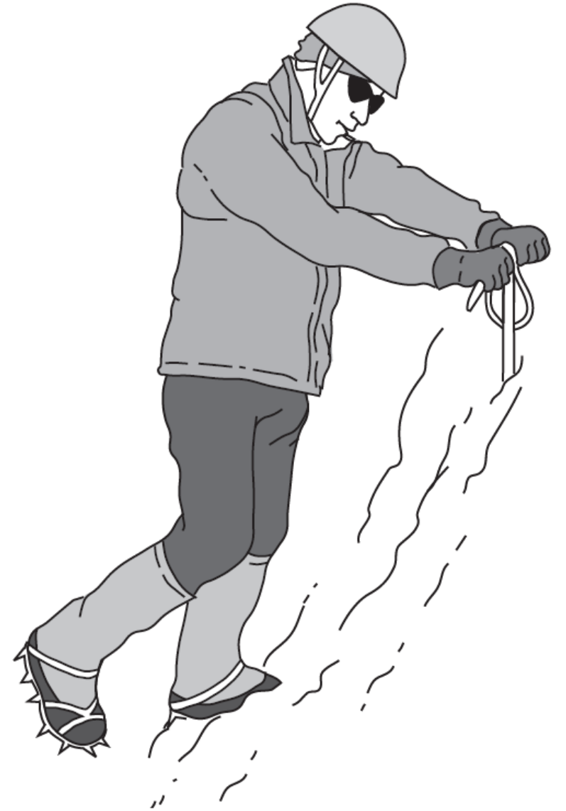
Fig. 16-23. Facing in (backing down): place ax low on the slope and don't lean in toward the slope.
