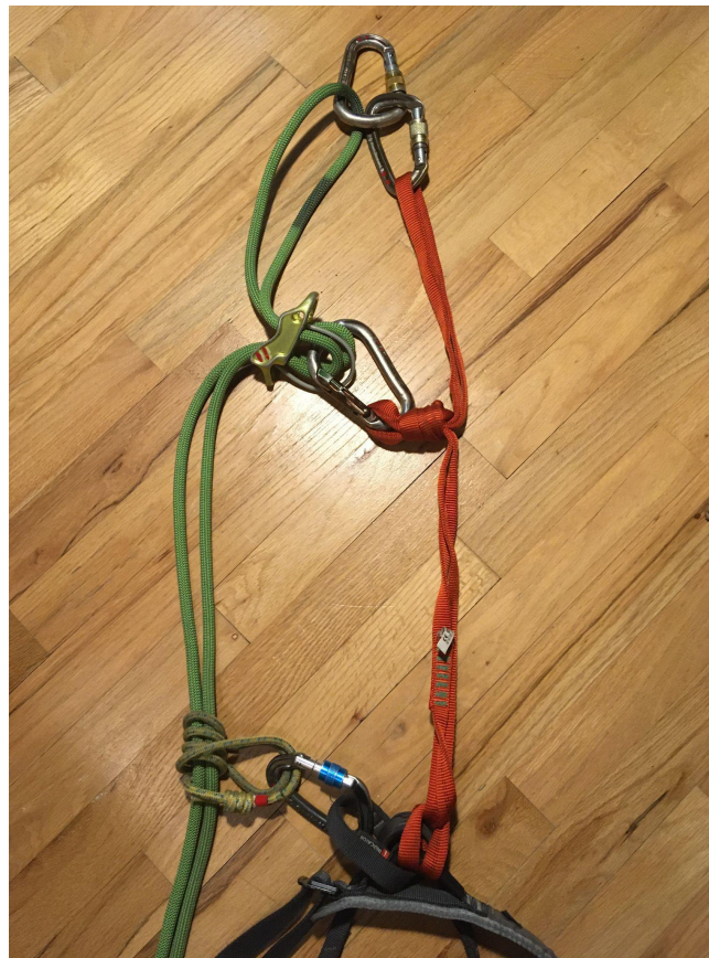
Anchor and extension with nylon sling with overhand on a big knot
