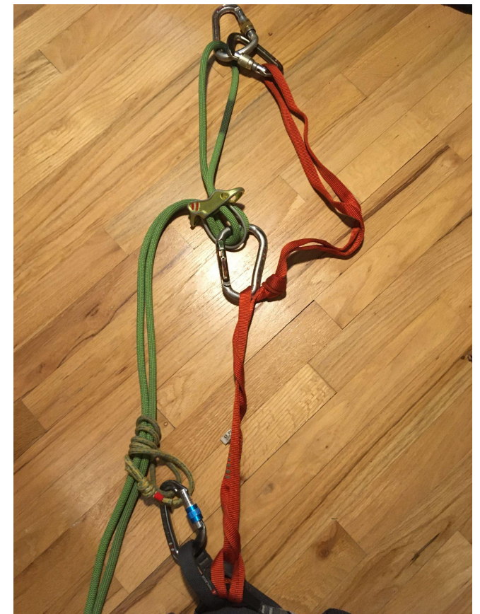
Anchor and extension with nylon sling with overhand knot
