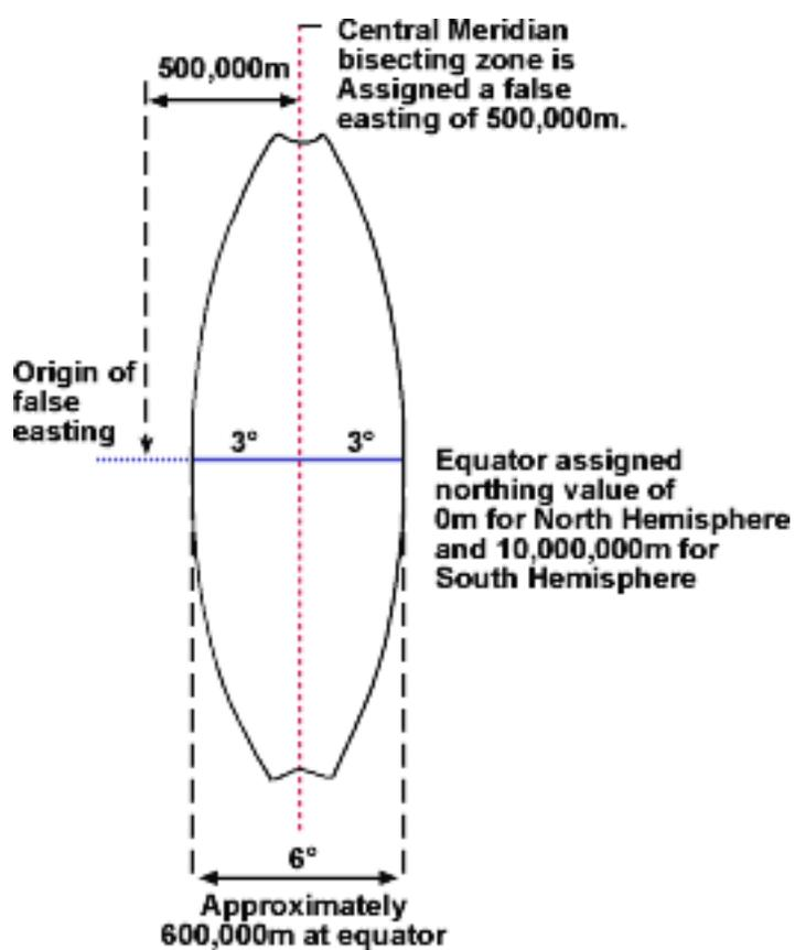
Any point can then be described by its distance east of the origin (its ‘easting’ value). By definition the Central Meridian is assigned a false easting of 500,000 meters. Any easting value greater than 500,000 meters indicates a point east of the central meridian. Any easting value less than 500,000 meters indicates a point west of the central meridian. Distances (and locations) in the UTM system are measured in meters, and each UTM zone has its own origin for east-west measurements.
