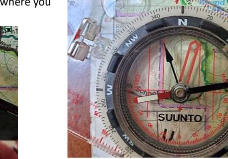
2. Rotate bezel so meridian lines line up with N-S lines on map (be sure that the N is pointing toward the top of the map)
