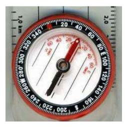
Keeping the compass flat and square to your body, walk forward while keeping 'red in the shed'. This is 'following a bearing', in this case along the West Tiger 3 trail.
