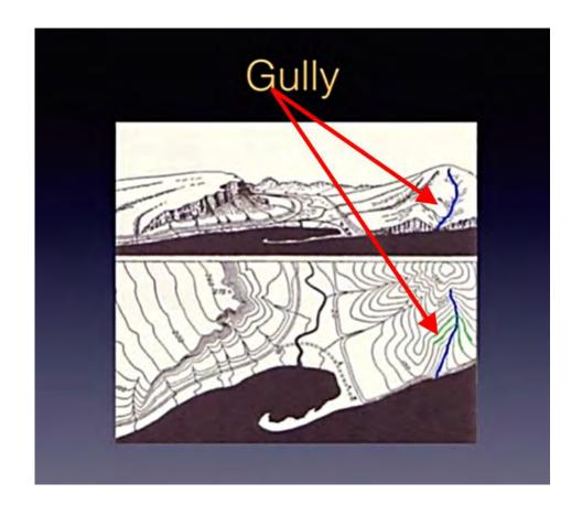
Creeks or rivers are usually great giveaways for the location of a gully or valley. The direction of flow (always downhill!) indicates what direction is uphill and downhill.
