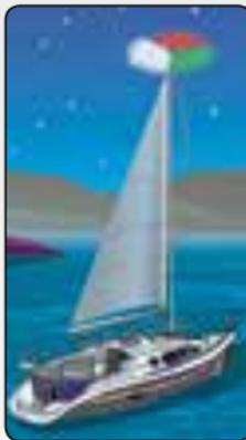
An alternative to the sidelights and sternlight is a combination red, green, and white light, which must be exhibited near the top of the mast.
