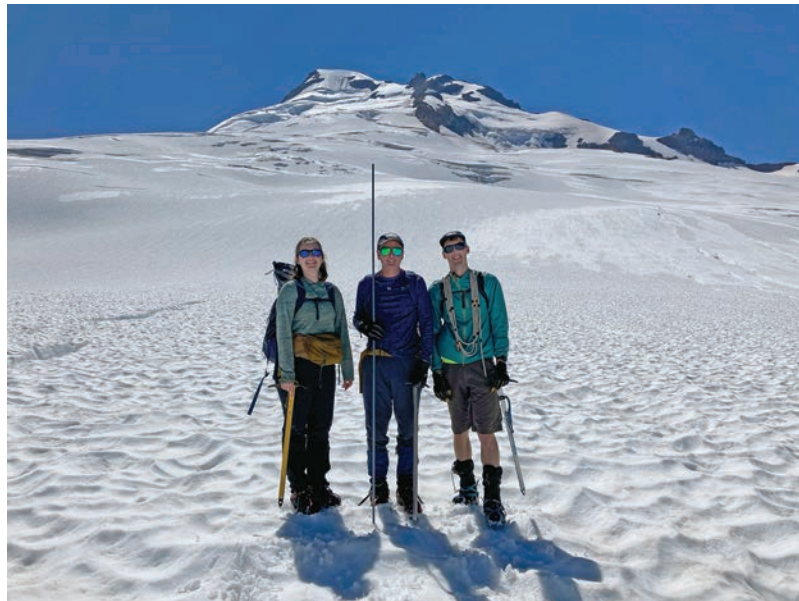
Left: Observing annual snowpack thickness on Rainbow Glacier in August 2024 via color variation in crevasse layers. The whiter layer is from the 2024 winter, and the browner layer beneath was deposited during the 2023 winter. Above: Jill, Mauri, and Ben Pelto on the Rainbow-Mazama Glacier Saddle using a snow probe to safely measure snow depth. Collectively, the family has spent 75 field seasons observing North Cascade glaciers.
